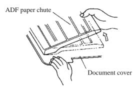
Figure 4.3 ADF paper chute setting
